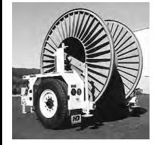
The Hogg & Davis, inc. Model T150 Cable Reel Dolly is an open yoke unit designed for low center of gravity reel hauling. It offers operating ease and simple maintenance. The 4" x 6", 1/2" wall tubular frame, super structure and heavy duty fenders and panels are integrated into a structurally strong and rigid unit designed for years of rugged service. It is backed by years of experience, knowledge and quality which Hogg & Davis, inc. is known worldwide for.
