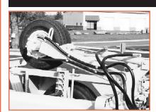
A hydraulically operated retriever arm is an available option for the TH40. It uses the towing vehicle's hydraulic circuit. It can be used for light duty stringing operations.
