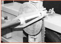
An optional reel brake is available to provide antiover-spin control necessary for pay-out operations.
