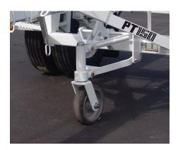
Idler Wheel – Setting the PT150 apart from the competition is its unique hydraulically actuated Idler Wheel. The double A-frame mounted assembly provides 360° swivel and ease of motion with its bearing mounted caster. The hydraulic pump is easily accessible at the curb side of the unit. Dual coil springs retract the wheel for towing.
