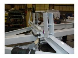
BOLSTER CHOCKS – Bolster chocks that don't get lost. We feature bolster chocks with built in winches that cannot fall off the bolsters. Each chock is attached permanently but easily moves around the end and down under and out of the way if necessary. Fifteen feet of 3/8" cable provides plenty of tie down capability for the fullest loads.
