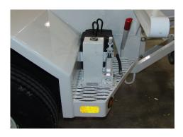
**PUMP** – The sturdy manual **hydraulic pump** is located at the curbside of the trailer. Easily accessible, even with a full load of poles, the pump actuates the hydraulic idler wheel for easy hitch adjustment for hook up. (Each trailer is provided with four wheel chocks, as seen behind the pump)
