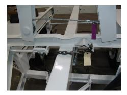
**CENTER POLE BINDER** – A unique feature of Hogg & Davis Inc. is the built in **over center chain binder** for the lead pole. Providing solid holding of the center pole allows greater load integrity and towing confidence. Successfully used for over 30 years by Hogg & Davis Inc. this feature helps the PT150 stand above the competition.
