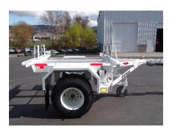
Cargo Trays – Optional removable cargo trays allow the PT150 to carry the hardware needed when the jobsite is reached. The trays are 62" long by 18" wide and 6" deep and bolt securely in place. Cut out type handles provide easy handling. Use one or both, these cargo trays provide plenty of room for hardware, insulators, connectors, etc., that you will need on the job.
