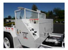
**Power Unit Conversion:** This is the basic conversion. Includes a completely new Tier 4 Yanmar diesel powered hydrastatic power unit rated at 24,000 lbs. of line pull. All new controls at the front and rear. Also includes a new power unit cylinder with integrated holding valve to move the power unit back and forth. Ready for your shop to install or send your unit to Hogg & Davis for us to do the conversion for you.
