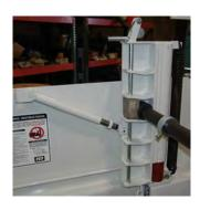
Bearing Mandrel Rack Conversion: Add this conversion to improve smoothness of payout and pulling operations while eliminating wear and tear on components. All metal to metal contact is eliminated with the use of Nylatron® mandrel bearings. Includes racks, bearings, bearing blocks and new reel mandrel.
