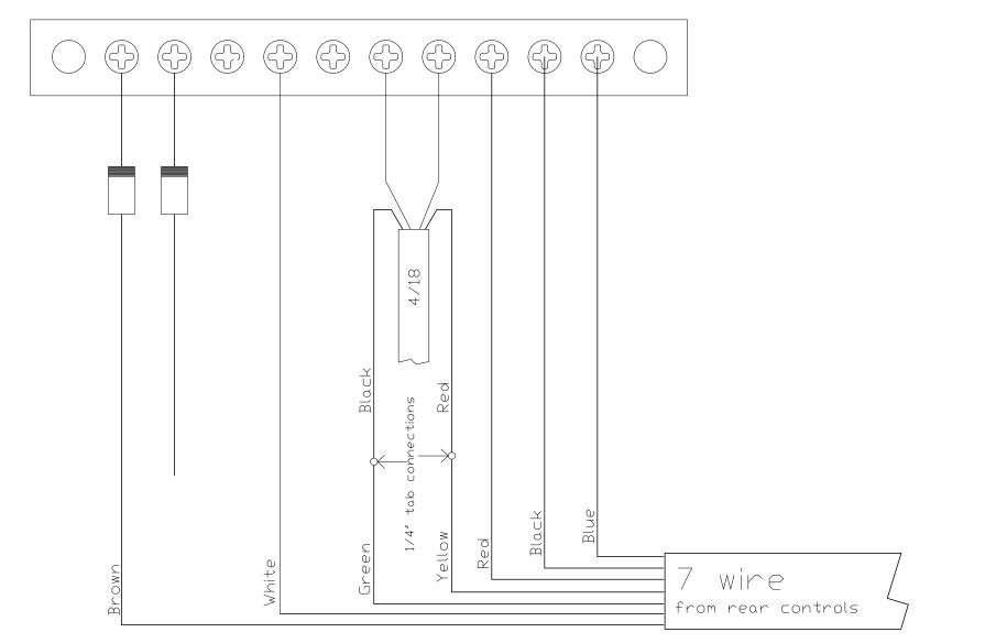
Tool Cirsuit equiped units require a 14/2 SJD to be run along with the 7 wire Level Wind equiped units require a 14/3 SJD to be run along with the 7 wire
