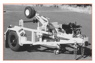
Increase the versatility of your R 40 by adding the **optional retriever.** This unit will provide approximately 1500-2000 lbs. line pull. The retriever utilizes the hydraulic tool circuit of your truck to provide pressure against the reel and rotation of the retriever wheel. This is a bolt-on option that can be easily added to the unit by your personnel.
